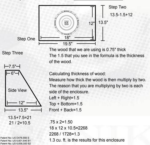
Calculating speaker enclosure volume is a five step procedure. (Make sure you do not forget to subtract the thickness of the wood and port displacement that you used.)
